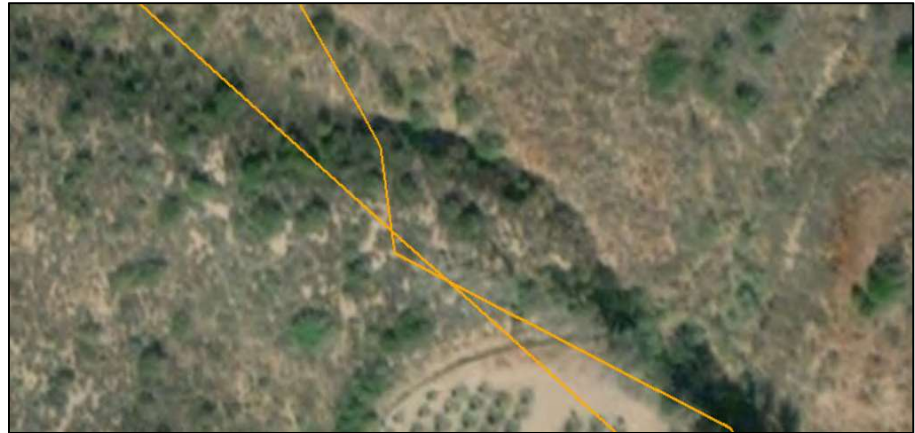
Figure P3-Example of Sliver in LAND and LANDOWNER Feature Classes for "Open Space" Polygon Features
