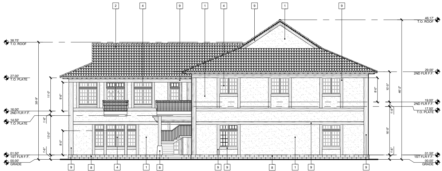
1 PARISH HALL EAST ELEVATION SCALE: 1/8" = 1'-0"
